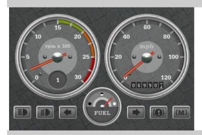
The tachometer (the large dial on the left) also indicates the current gear as a figure in the gray circle at the bottom of the dial. On this example, we are in 1st gear ('1').
