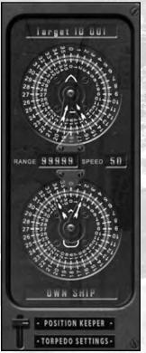
The great advantage that U.S. torpedo data computers have over those of other nations is the Position Keeper (PK). This unique device estimates the target data based on the initial values entered by the user. It computes the target movement in relation to your submarine, taking into account your own ship movements.
