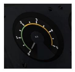
The power handle on this locomotive primarily controls the rotation speed of the diesel engine. An automatic load regulator controls the power delivery so as not to overload the engine. When the engine rotates faster, more electric power is delivered to the traction motors, and vice versa. Power delivery can be monitored on the main ammeter, pictured above.
