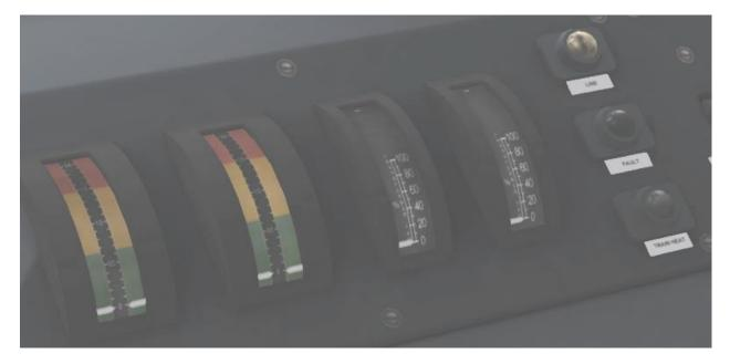
The present notch setting is displayed on the notch meters (on the right) as a percentage of maximum. Thus on this class of locomotive, Notch 39 appears at 100%. The left-hand of the two notch meters shows the notch setting on this locomotive, while the right-hand one is supposed to display the setting on the second locomotive of a pair - however, fitters are still tracing a persistent fault in this equipment, which disables the second meter.
