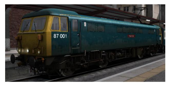
The Class 87 locomotive was purpose-built for hauling fast express trains on the West Coast Main Line, especially on the steep gradients of Shap and Beattock, as a straightforward development of the established Class 86. Nominally rated for a very impressive 5000 horsepower - and with even more available on a short-term basis - a Class 87 can cruise at 110 mph indefinitely if line conditions permit.
