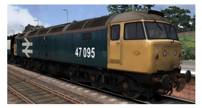
The Brush Type 4 locomotive, as the Class 47 was originally known, is a powerful mixedtraffic locomotive powered by the well-regarded Sulzer 8LDA12-B diesel engine. With a maximum permitted speed of 95 mph, over 2500 horsepower on tap and roughly 120 tons of adhesive weight on six axles, the class is highly versatile and was built in large numbers during the 1960s. Dozens of surviving examples are still used on the mainline network well into the 21st century.
