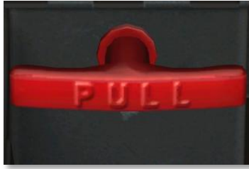
Figure 62: Landing Gear Fairing Door Emergency Release Handle
