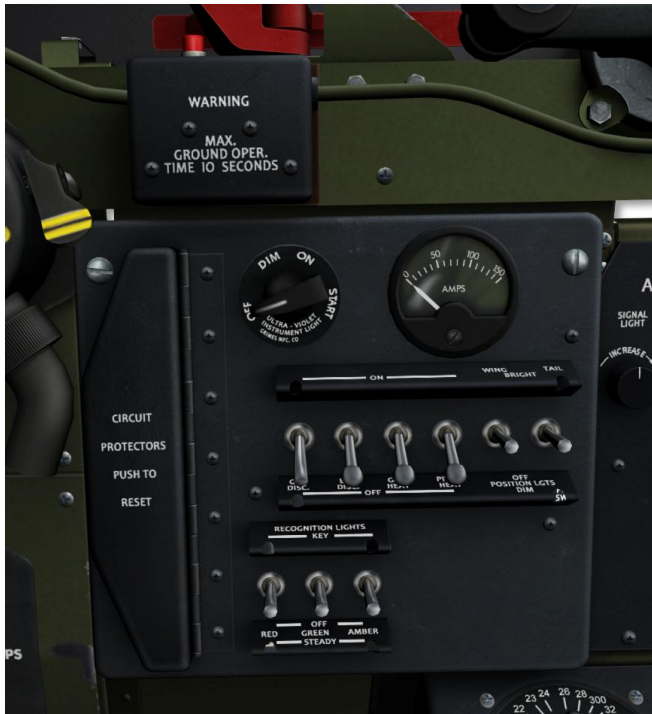
Figure 25: Electrical Control Panel
