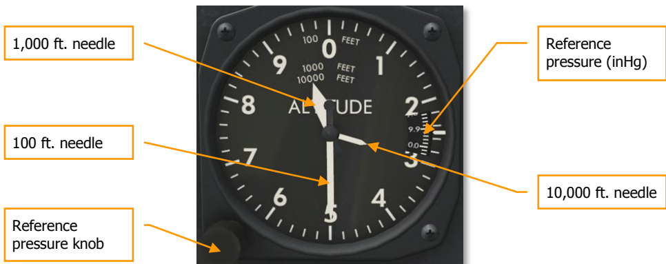
Figure 44: AN5760-2 Pressure Altimeter indicating 29,500 ft.
