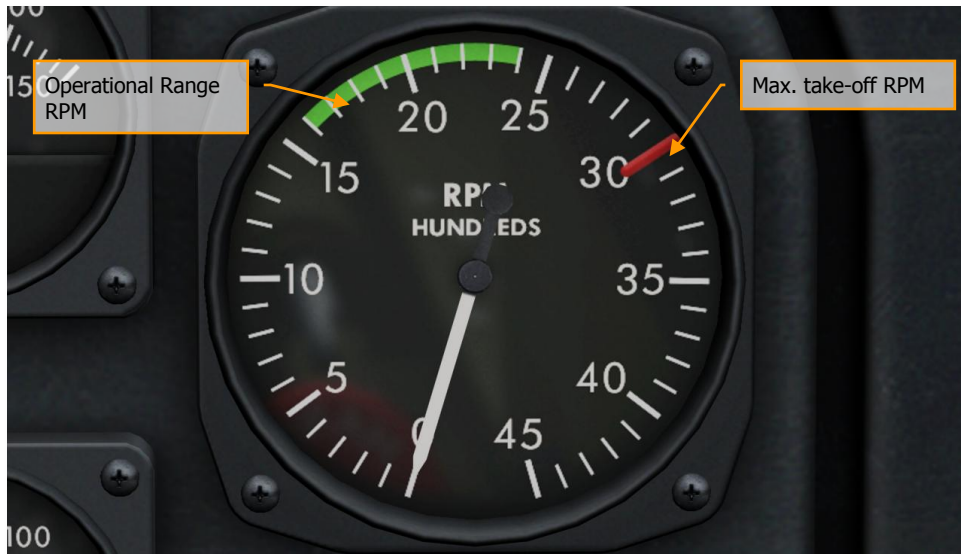
Figure 84: Max. take-off RPM 3000. Operating Range 1600...2400.
