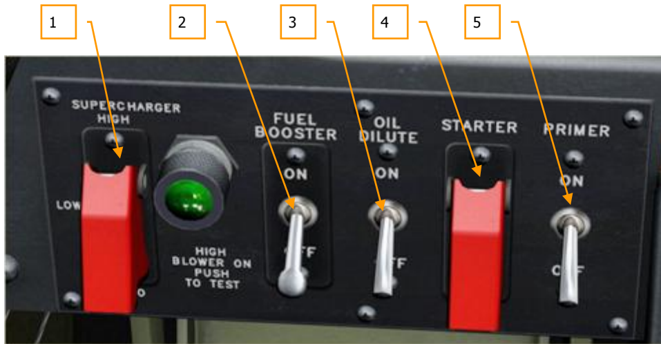
Figure 58: Engine Control Panel
