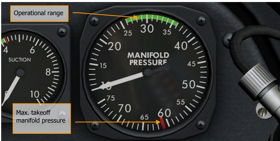
Figure 82: Max. takeoff manifold pressure – 61 in. HG (155 cm HG) (red mark). Operating range 26...36 in. HG (66.04 - 91.44 cm HG) (green zone).
