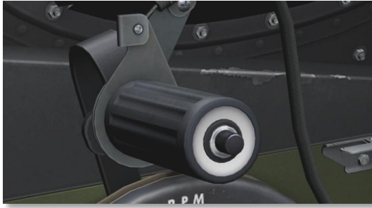
Figure 94: Throttle Control handle with twist grip
