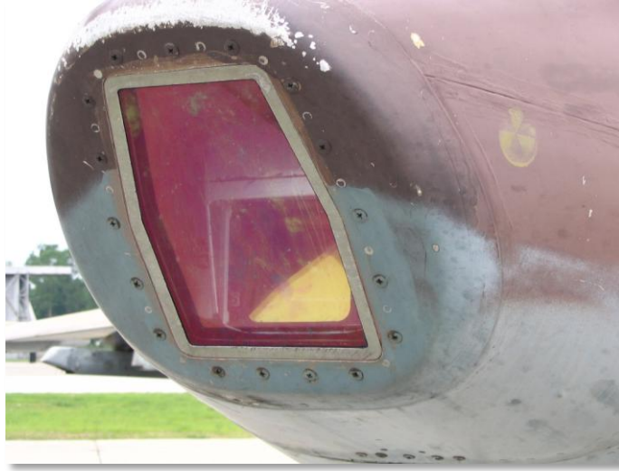
Figure 22. Nose of Su-25 with laser rangefinder "Klen"
