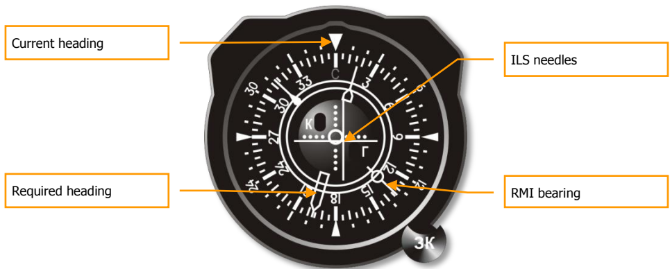
3-42: Horizontal Situation Indicator (HSI)
