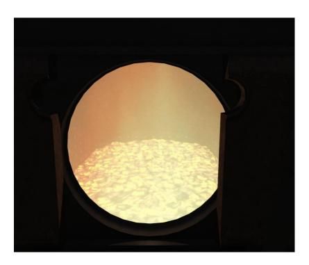
Coal level high > 83% 982 lbs The grate is deeply covered with the coal's centre almost up to the 1<sup>st</sup> row of rivets on the back wall.
