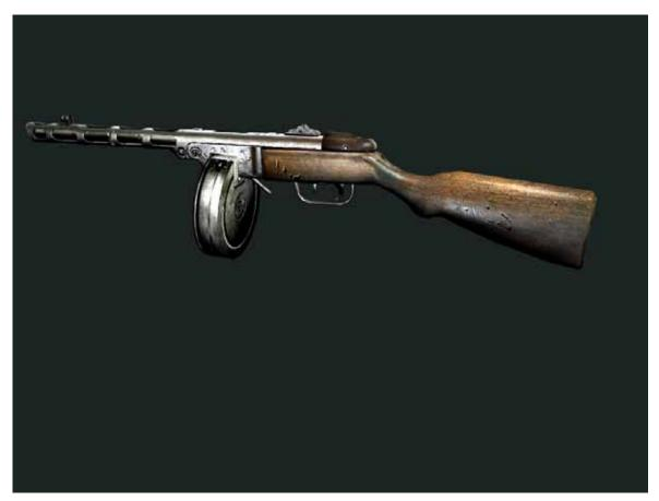
**PPSch-41 Submachine gun.** (Russian model) Technically this gun consists of a barrel and breech block cases connected with a joint, or with a catch, located at the back of the barrel case, if the gun is assembled; a case of launching mechanism, located in the stock under the breech block case; a wooden gun-stock with a butt. This weapon during the Second World War proved to be reliable and powerful and till now it is adopted in the German active forces and used by Russian guerrillas.
