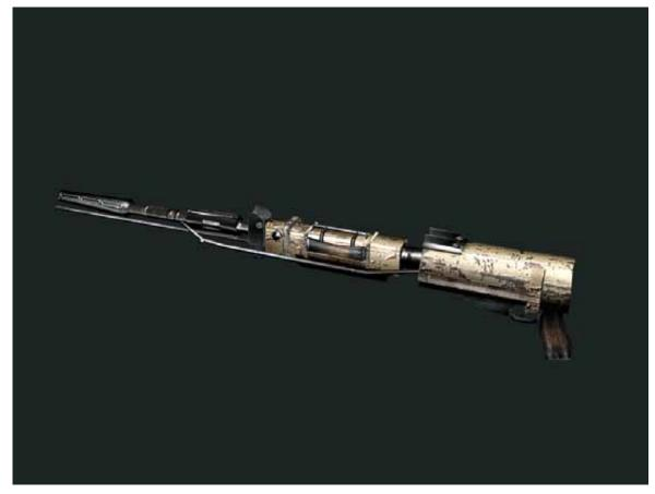
"Phoenix" Flamethrower. The complete set includes the container with an explosive mixture and a high-pressure cylinder for compressed air, which make the single unit, the feeding hose and the trigger. Compressed air is supplied simultaneously to both containers through the reducer and the reverse electromagnetic valve. The transformer increases the voltage up to 20000 volts and connects it to the spark device, which ignites the mixture.
