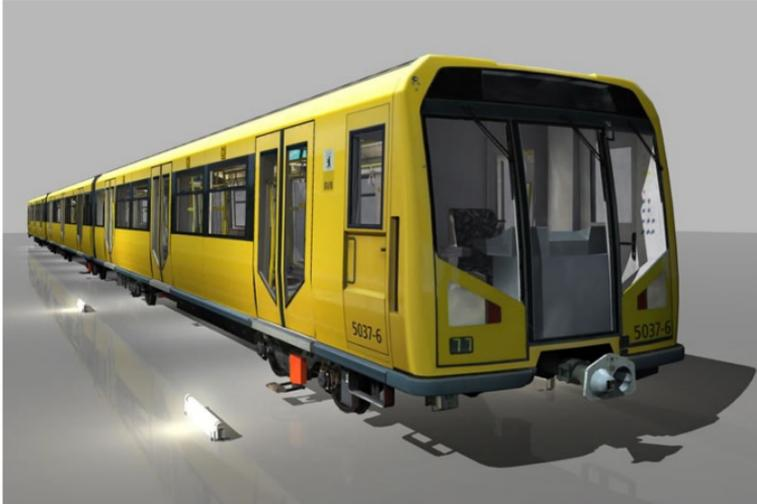
The H 01 is the most modern vehicle of the Berlin Underground system. This wide gauge train was built between 200 until 2002.
