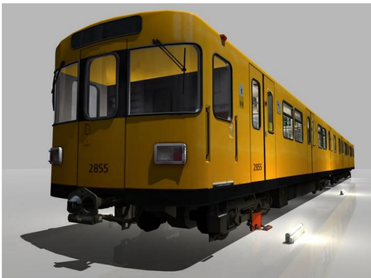
The F series started of in 1974 as the (F74) and was continually developed from there. The F90 was built in 1990 and 1991. The structure and design of this vehicle compared to the H series is rather plain though it represents the timeless elegance of the 70's and 80's.
