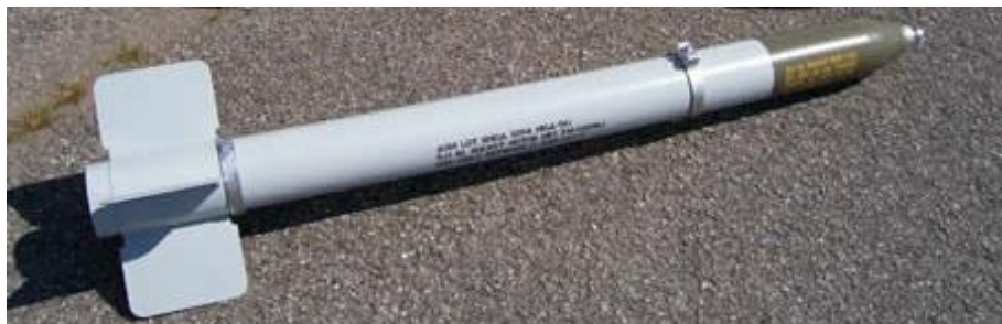
Figure 1.18. Unguided 127 mm HVAR (High-Velocity Aircraft Rocket)
