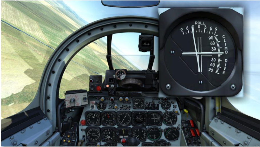
Figure 11.2. LABS Roll Indicator Reads 35° LH Roll
