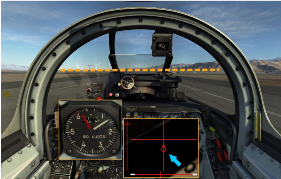
Figure 8.2. Position of the flight stick and canopy before detachment of the airplane from the runway
