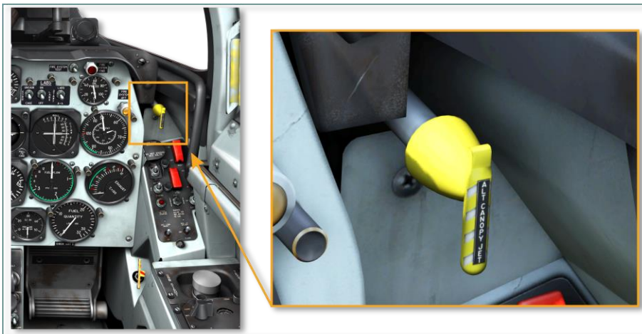
Figure 3.11. Canopy alternate emergency jettison handle
