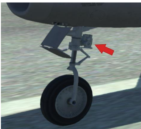
Figure 4.5. Nose wheel steering mechanism
