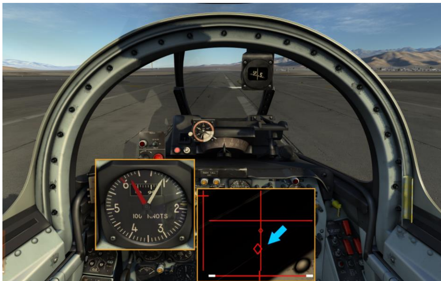
Figure 8.1. Position of the flight stick, when the speed is 20-30 knots lower than required for nose wheel lifting
