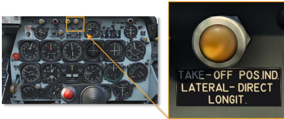
Figure 5.1. Take-off trim position indicator light
