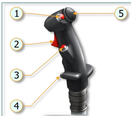
Figure 4.3. Flight control stick grip with buttons
