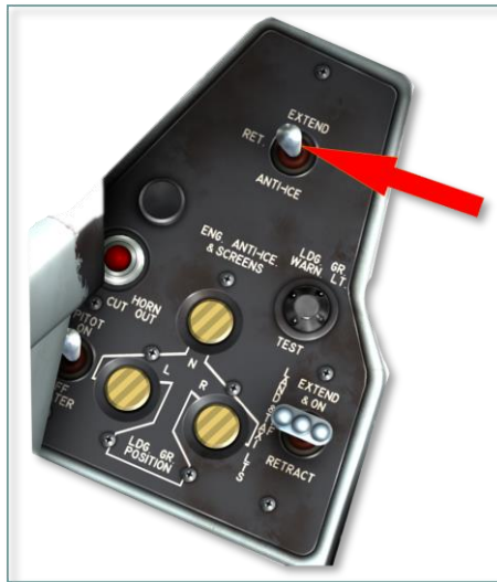
Figure 5.9. Engine protection switch
