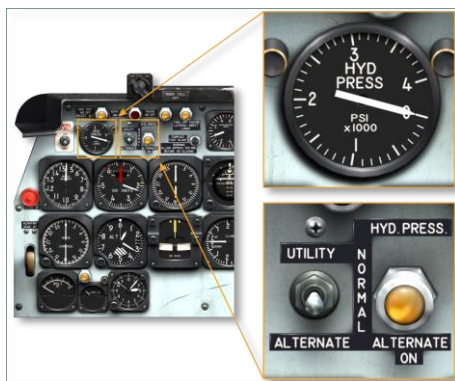
Figure 5.6. Hydraulic system indication and controls
