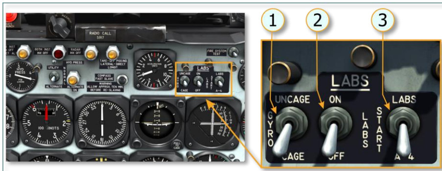
Figure 6.9. LABS Switch Panel
