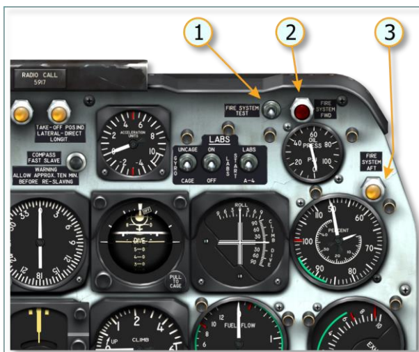
Figure 5.10. Fire indication system
