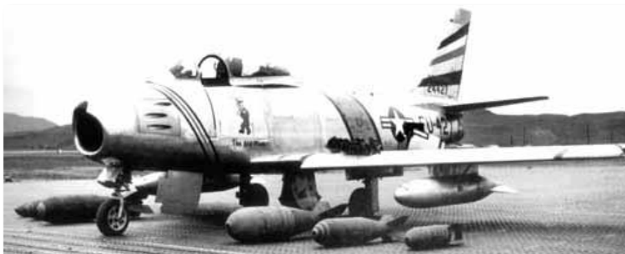
Figure 1.26. F-86F displaying bomb load variants
