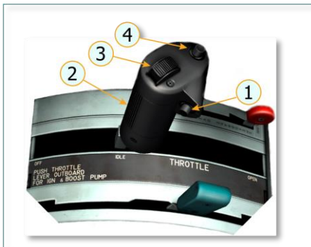
Figure 4.4. Controls on engine throttle grip
