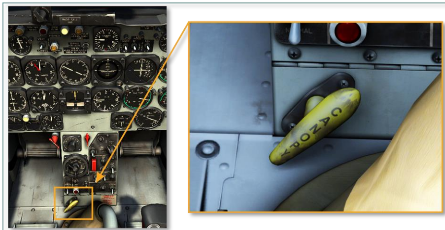
Figure 3.9. Canopy declutch handle
