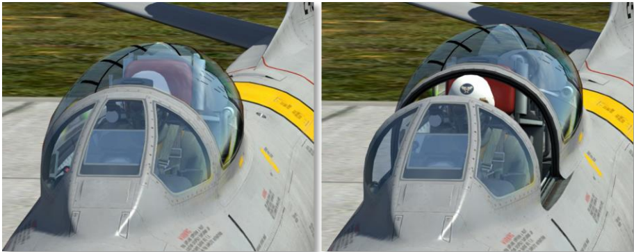
Figure 3.8. Closed (left) and opened (right) canopy
