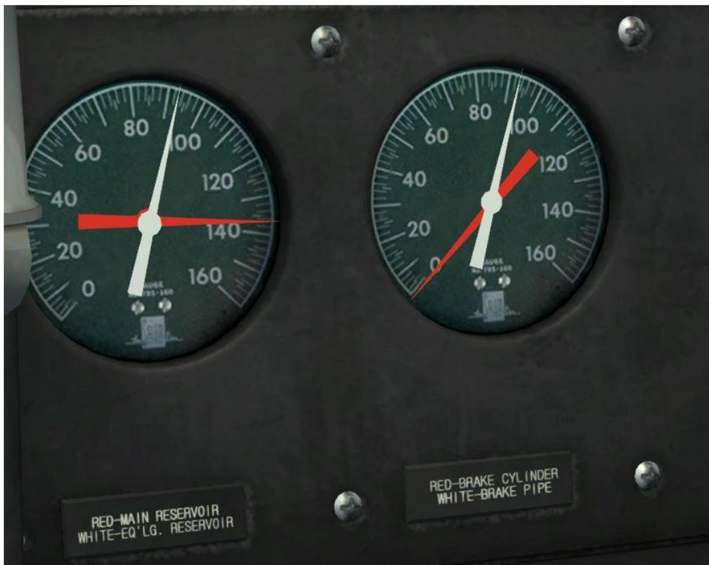
In the example above the brakes are released and both the Equalising Reservoir gauge and Brake Pipe gauge show 90psi.
