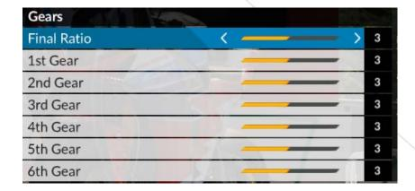
Lowering the final ratio gives you more acceleration, increasing it gives you greater speed. With a lower ratio the engine responds much faster when you accelerate or decelerate, so the bike will be more aggressive and you will have to ride more carefully. By using very high ratios you will be able to reach greater speeds while avoiding abrupt reactions when the bike is accelerating. Remember that you can change your final ratio if you are not satisfied with the difference between each gear.
