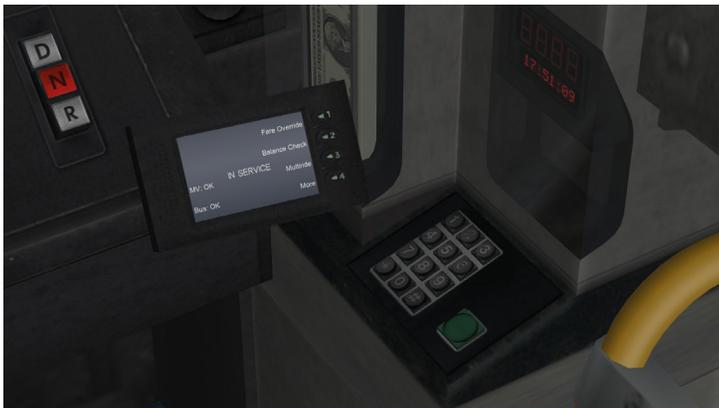
The external input device is located left of the farebox. It displays the login status and offers the possibility to override a fare payment or check the current balance.
