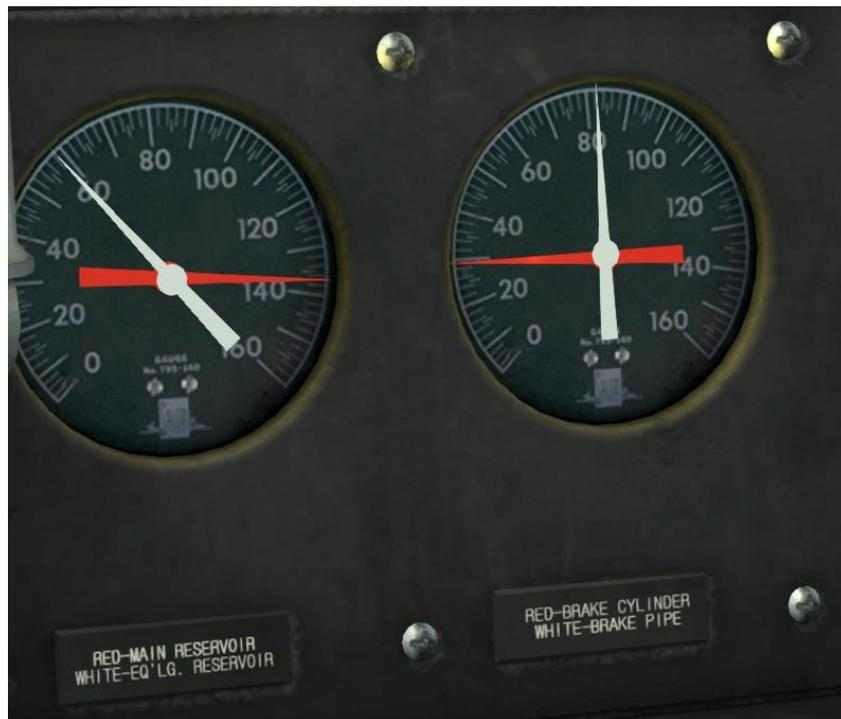
By moving the Train Brake lever further forwards (after a brief pause) the pressure in the Equalising Reservoir will rapidly reduce and show the 'target' Brake Pipe pressure. Air will be released from the system until the Brake Pipe pressure matches that of the Equalising Reservoir and how rapidly the air is released is dependent upon the train length. In the picture above the Brake Pipe pressure is dropping while the Brake Cylinder pressure is increasing.
