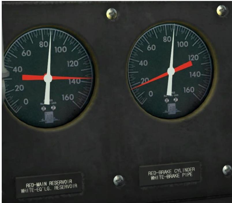
The Train Brake lever has a series of distinct stages to aid the driver. From the release position the first stage produces an almost instantaneous initial reduction of 6psi.
