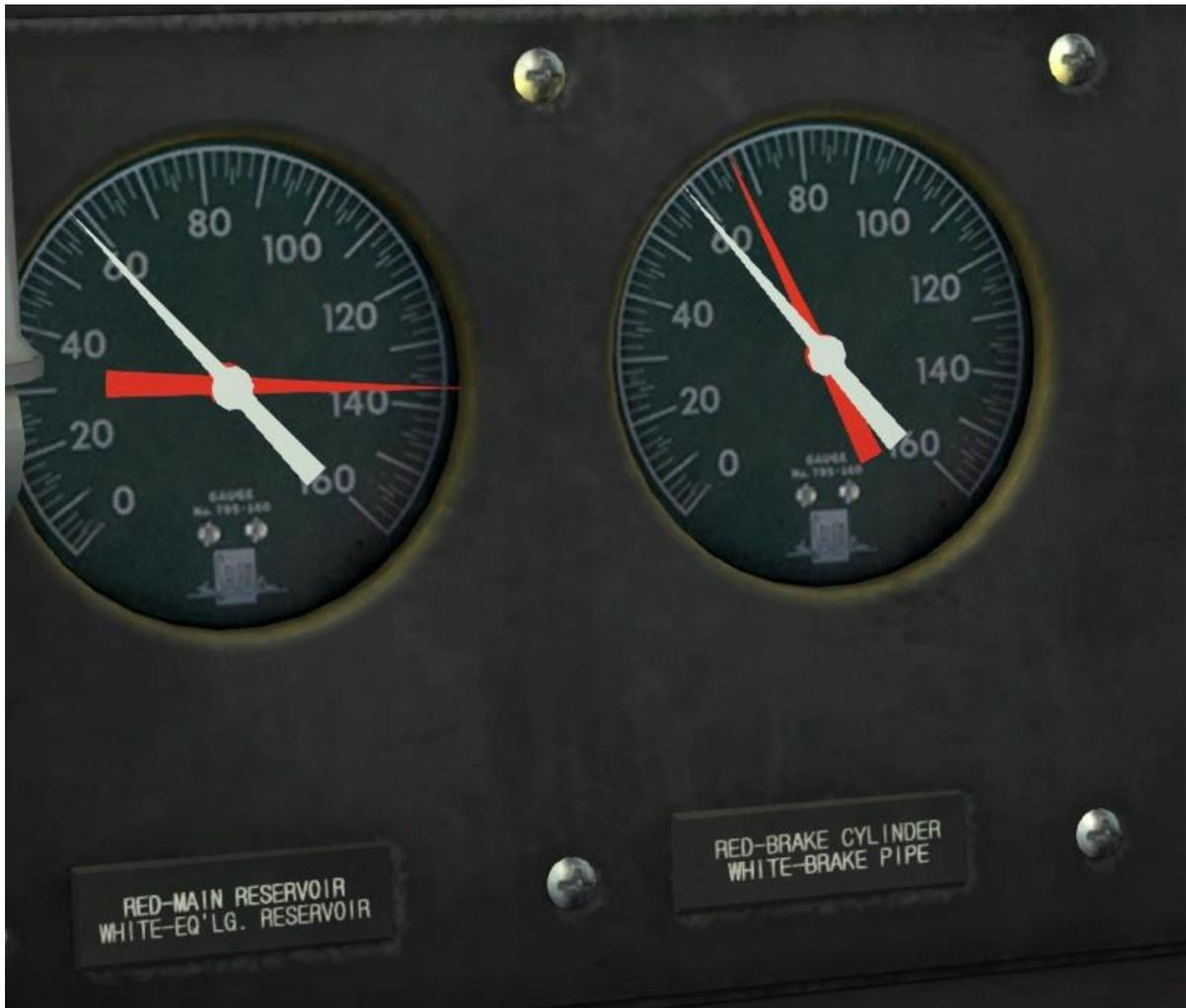
After a period of time the Brake Pipe pressure matches that of the Equalising Reservoir and the desired brake application has been made.
