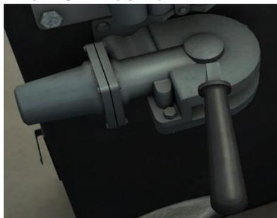
**\*\*If an emergency brake application is required a brief pause is required before the Train Brake lever can be moved between its maximum application setting and the Emergency Brake setting to avoid accidental application.\*\***
