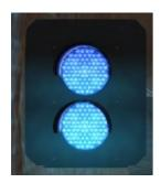
Re-apply power and release brakes before reaching this signal.
