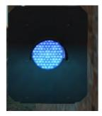
Start applying brakes before reaching this signal.
