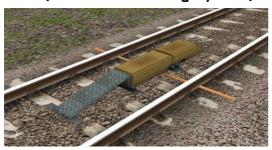
AWS is provided to give train drivers in-cab warnings of the approach to signals, reductions in permissible speed and temporary/emergency speed restrictions, and to apply the brakes in the event that a driver does not acknowledge cautionary warnings given by the system.
