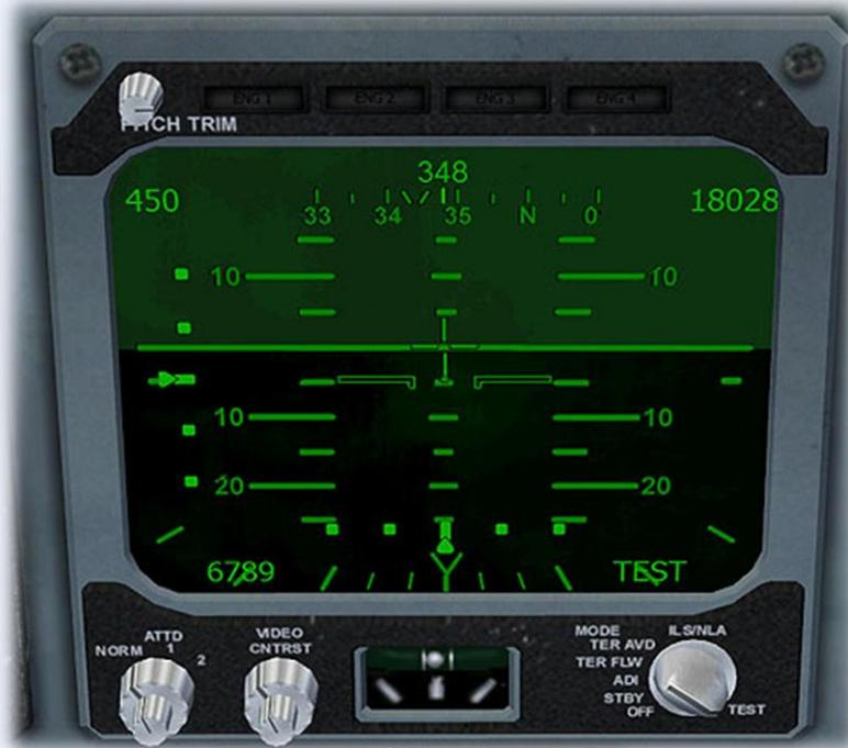
TEST mode displays all available functions, along with the text 'TEST' in the bottom right corner.
