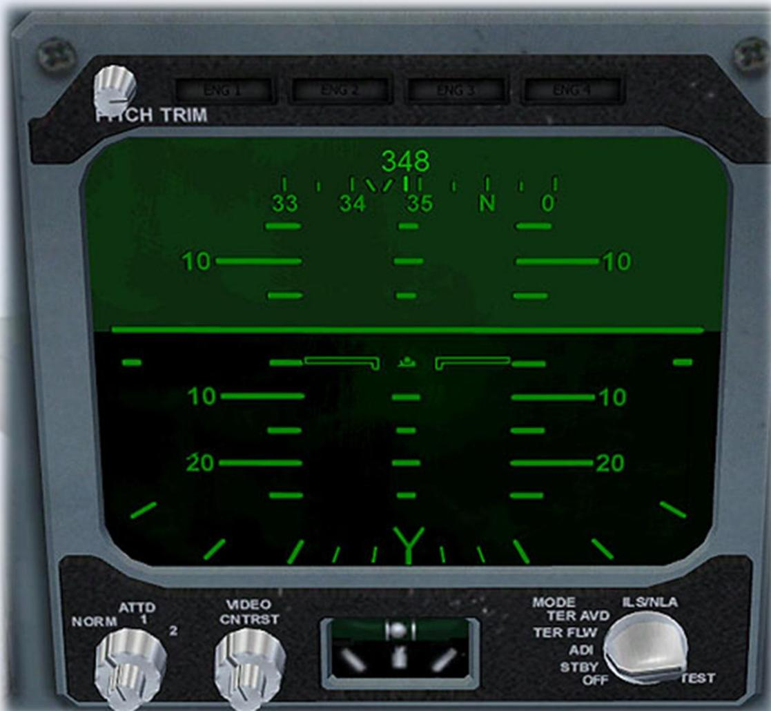
The VSD can be dimmed for night operation by using the contrast knob to the left of the turn and slip indicator. The default mode is ADI. This displays basic information. Central to the display is the pitch and roll ladder. This acts as an artificial horizon. Along the top of the display is a progressive gyro heading indicator, above which is a digital readout of the current exact heading.
