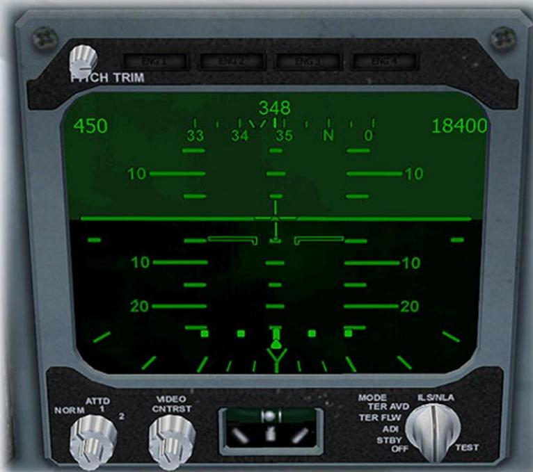
LS/AILA mode displays a digital course deviation indicator along the bottom of the ADI. If a glideslope is available, a similar glideslope deviation indicator will display along the left side of the ADI.
