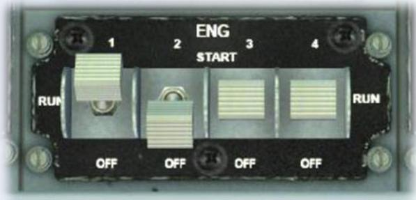
Left-clicking a control switch will cause it to enter the START position, and spring back to RUN after the engine start sequence has been initialised.
