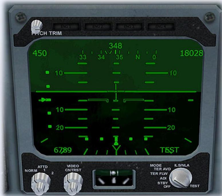
TEST mode displays all available functions, along with the text 'TEST' in the bottom right corner.
