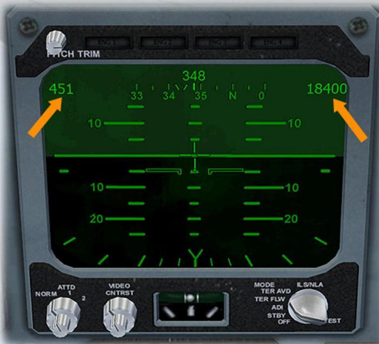
TER FLW mode builds on the ADI by adding a digital speed readout in the top left corner, and an altimeter readout in the top right corner.
