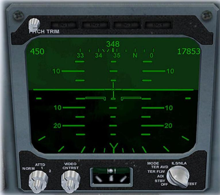
TER AVD mode is like TER FLW mode, except the altimeter readout is from the radar altimeter rather than the usual indicated altitude.
