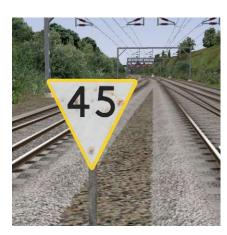
These signs provide advance warning of a reduction in permissible speed ahead. Permanent AWS Ramps (Automatic Warning System) are often installed in conjunction with these signs. In these cases the driver must cancel the AWS warning when triggered on approach to these signs.
