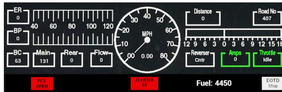
Once the emergency brake has applied and the "PCS OPEN" indicator is showing you will need to let the train stop and then follow the PCS Reset procedure for the AC4400CW to continue. This is detailed in a following section of this document.
