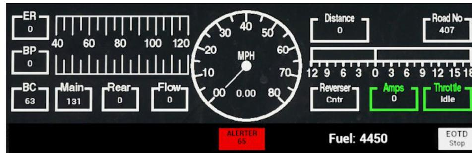
This indicator shows "ALERTER 65". The 65 is the countdown timer so that you can always see it, if you are travelling over 5mph then this will begin to count down and once it gets to 5 the alerter will sound and must be responded to by pressing the Acknowledge button on the desk, the Q key on your keyboard or the B button on your Xbox controller before the counter finally reaches zero.
