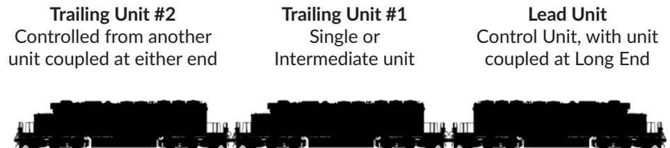
In this example, the light switches are set up as described in this three locomotive consist.
