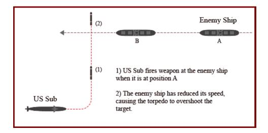
One way to hedge against target zigs is firing multiple torpedoes in a salvo, or spread:
