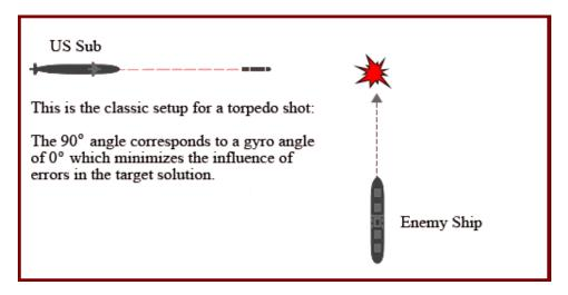
The accuracy of the solution is dependent on several factors: Sudden movements by you or the target may invalidate the solution causing your weapons to miss. Therefore unguided torpedoes can easily be defeated by a manoeuvring target. This has been made into standard doctrine, and therefore all surface groups will make periodic course changes, or zigs, to throw off any skipper trying to ambush them.
