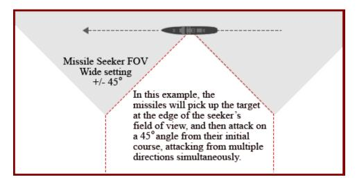
Due to the ranges at which missiles are commonly used, an important consideration is the activation distance from the target. A short distance means less time for the enemy's defences to react, but over large distances the enemy may have zigged or moved too far, causing the weapon to miss. Once you fire the missile, it is on its own - you cannot correct its course in-flight like you can with a torpedo.
