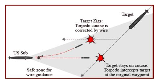
Weapons can be guided either by updating the activation point if the weapon is still in the run-to-enable phase of the torpedo run, or by directly steering the weapon if it is active. Steering an active weapon will override any terminal homing, and so is useful for guiding the weapon away from decoys or overriding a weapon that is homing on the wrong target.
