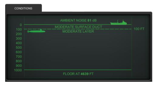
The Conditions display lists the current ocean ambient noise level, the depth and strength of a layer (if one exists), the strength of a surface duct (if one exists) as well as the depth to the ocean floor. In addition, your submarine's depth is plotted (if above 1000 ft) and if your current contact's solution is high enough, that contact's depth is also shown.
