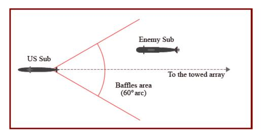
A towed array is not affected by the rear baffles as the listening device is towed far behind the vessel. However the towed array has a narrow blind spot forward as the noise from the submarine ahead masks incoming sound.
