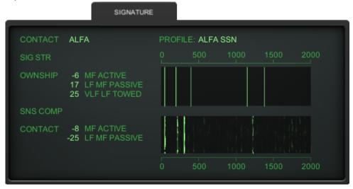
Use **F6** (Shift 6) or click on the Signature tab in the bottom right to open the Signature Panel and view the current contact's sound profile (lower panel). The upper panel contains a database of known vessel profiles for comparison. Following the vessel name is the designation for that type of vessel, see Reference section for a list of ship designations.
