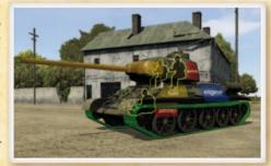
Vulnerable points are its tracks, main gun, engine, fuel tank and ammunition storage. The position of these points can differ in various types of tanks. However, on heavy tanks they can be well-enhanced with thick armor.
