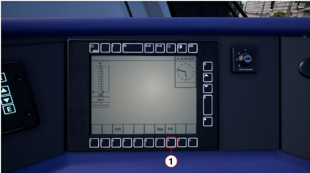
2. The display will present a representation of the trains in the consist and the destinations that are currently set, labelled 'ZUG 1', 'ZUG 2', etc. Press the '2' button (2) which is labelled 'Rout. Eing.' to set the destination.
