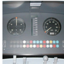
MFA20 with the LZB80 display in the ICE 3
