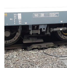
Train magnet passes over track magnet
