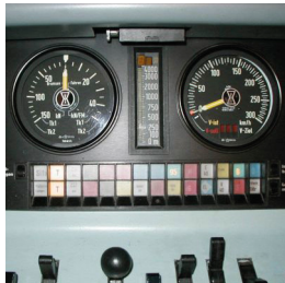
MFA8 with the LZB80 display in the ICE 1
