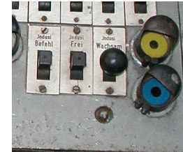
Indusi I54 installation with command, release and vigilance buttons and the two light indicators
