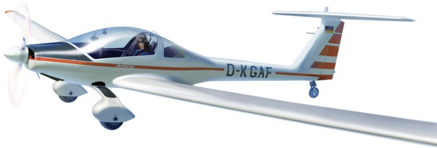
The Hoffmann H36 Dimona is not your regular small aircraft. It is in the rather exclusive class of touring motor gliders; aircraft that are a cross between motor aircraft and gliders. They got the long wings of a glider but a standard (though often rather small) aircraft engine. You can either use them as a normal aircraft or switch off the engine and glide for a while.
