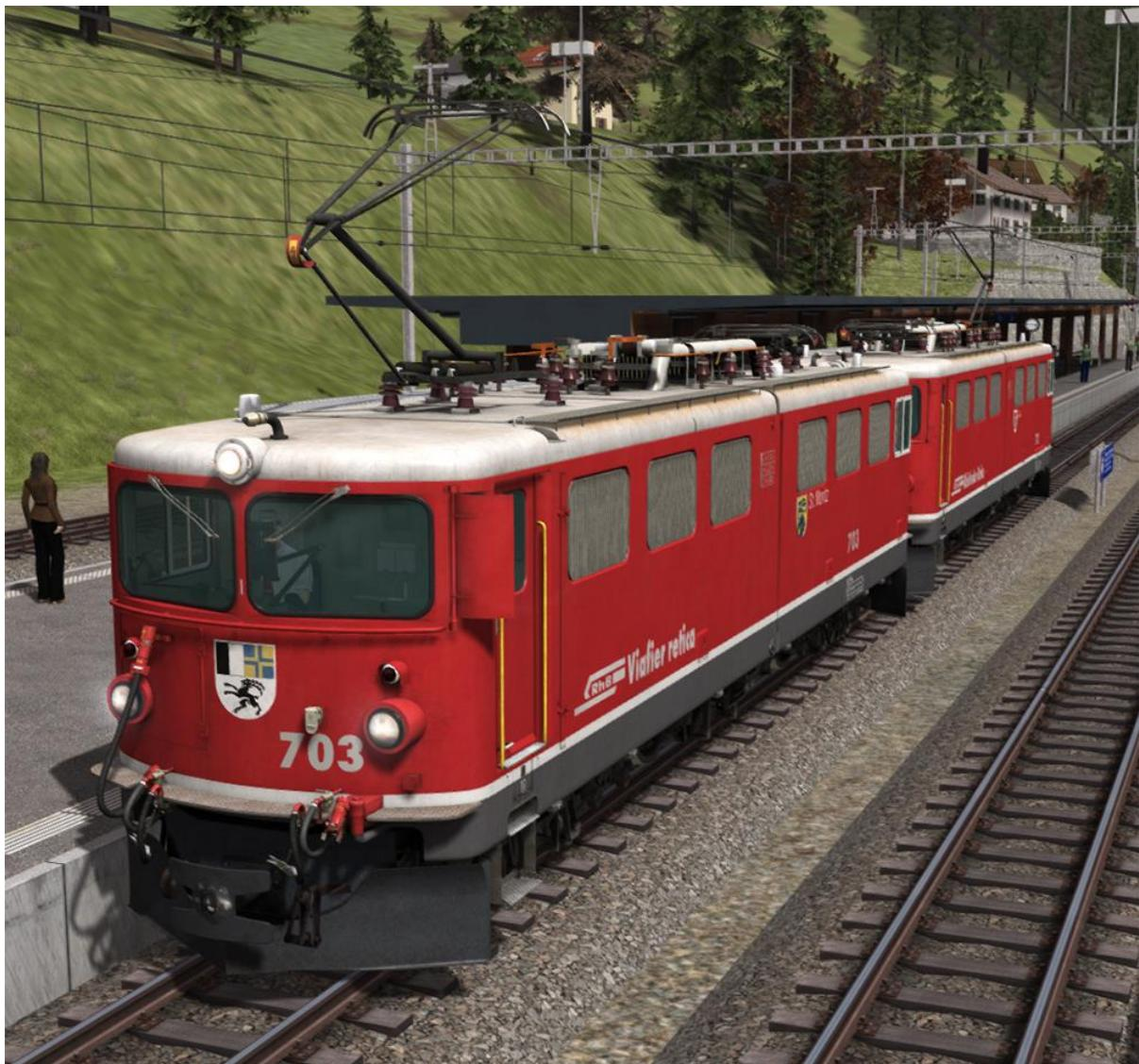
When operating Ge 6/6 II locomotives in pairs the automatic multiple working mode will be activated. This mode enables the front pantograph on the leading locomotive for use instead of the rear pantograph. Once uncoupled the locomotives will return to standard operation.
