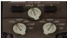
Open up the pedestal panel (**Shift+2**) and move the left **FUEL CONTROL** switch to the **RUN** position.
