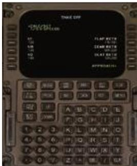
Another feature in the FMC is the ability to calculate and display the V speeds and approach speeds for the aircraft at its current weight. By pressing the 'TOFF/APR' button you will see this page.
