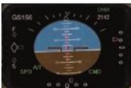
As the magenta indicator reaches the middle mark, the aircraft will pitch down, beginning the final descent into the airport. If the aircraft is stable, and the conditions favourable, you should be maintaining a descent rate of approximately -700 feet per minute.
