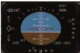
The magenta bug should now remain above the centre marker, indicating that the aircraft is correctly positioned on the localiser.
