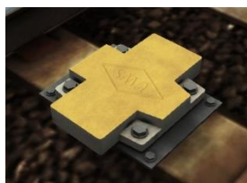
A Transponder on the track
