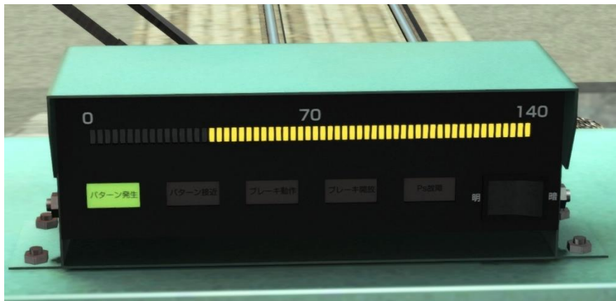
ATS-Ps speed pattern generated (train stopped)
