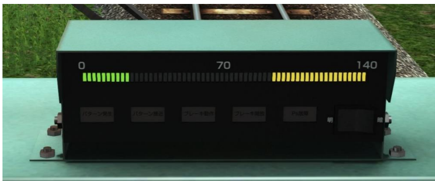
ATS-Ps speed pattern is not generated.
