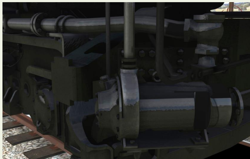
Figure 18: ESI Centrifugal Pump
