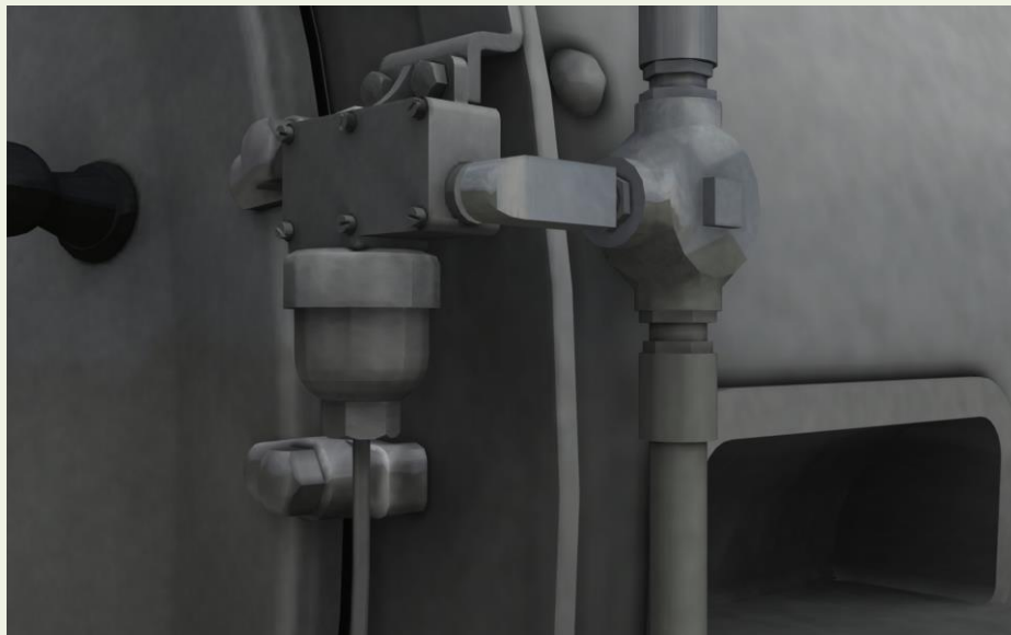
Figure 16: ESI Overflow Sensor
