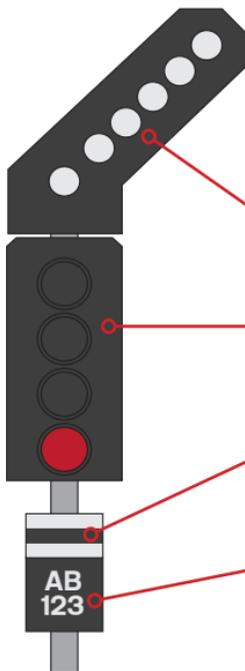
British colour light railway signals consist of one or more physical components or modules that form the basis of advising the driver on the state of the route ahead. The components are, from top to bottom:
