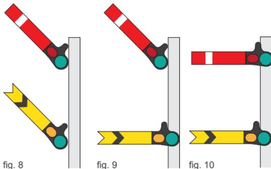
The signal on the left (fig. 8) both arms display a Clear aspect, so it is safe to proceed past this signal into the next block. This signal also advises that the next main signal is also displaying a Clear aspect, so it is also safe to proceed into that block too.
