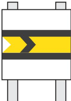
The Fixed Distant Board replaces the role of a controllable distant signal and essentially is regarded as a Caution aspect. This is therefore advising you that you may pass this board but the next signal will be at Danger. These boards are typically used on lightly-used routes and reduces the overall cost of signalling.
