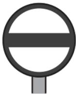
The horizontal band denotes the next main signal is displaying a stop aspect. You should be prepared to stop at the next signal.
