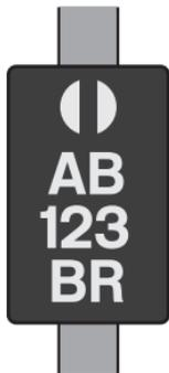
The upper part of the identification plate employs a form of code that advises the driver on what type of signal is deployed. In this instance, a three aspect banner repeater.
