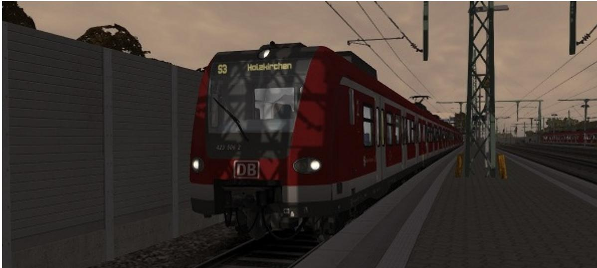
The Class 423 is an Electric Multiple Unit (EMU) made for the S-Bahn commuter networks of Germany (Munich S-Bahn, Cologne S-Bahn, Frankfurt S-Bahn and Stuttgart S-Bahn).
