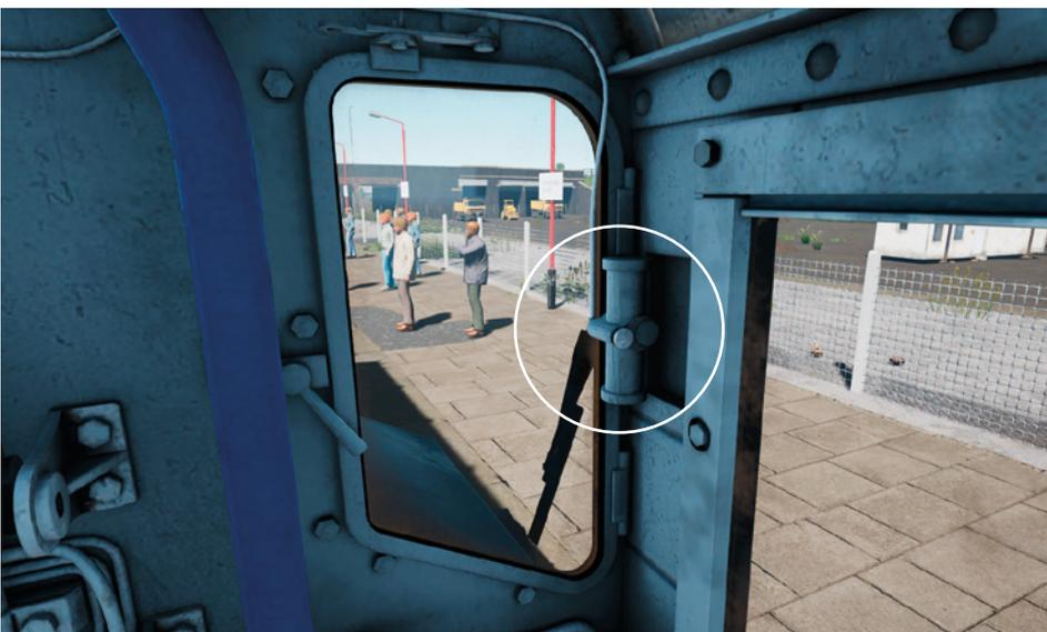
Use the button on the wiper motors to operate the windscreen wipers. They are variable speed.
