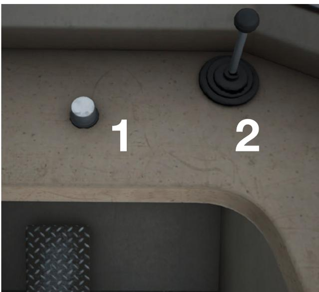
1. AWS alarm acknowledgement button – press to acknowledge the AWS alarm.
