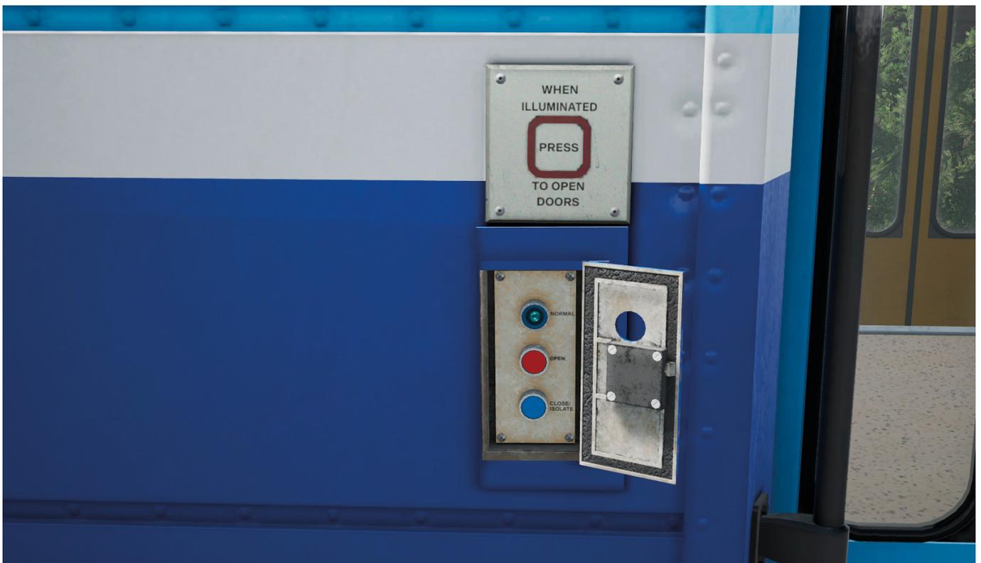
Inside the panel you will see three buttons. Press the red OPEN one to open the doors.
