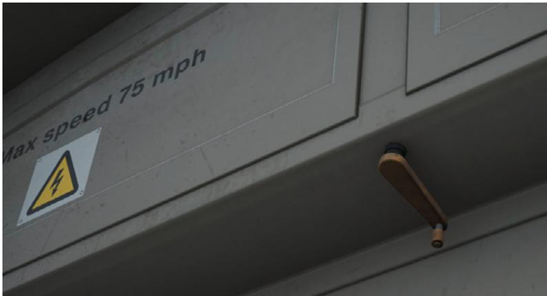
Rotate this handle to change the destination names in the exterior panel.
