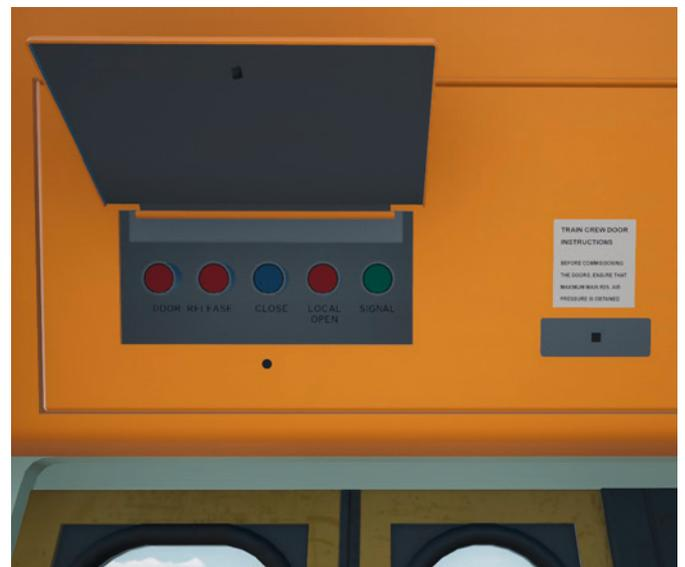
To **ONLY** open the door which you are standing next to, press the red LOCAL OPEN button. All the other doors will stay closed and locked. If you want to open **ALL** the doors on the platform side, press the two red DOOR RELEASE buttons.
