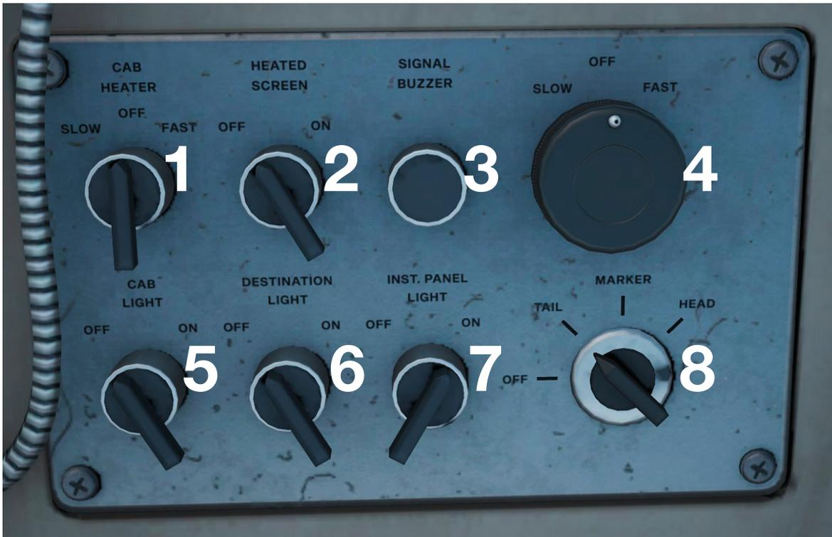
1. CAB HEATER – move the switch as required (SLOW/OFF/FAST).
