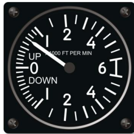
Figure 30. Vertical Velocity Indicator
