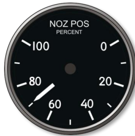
Figure 34. Engine Exhaust Nozzle Position Indicator
