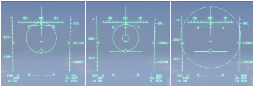
Figure 52. Vertical mode AIM-7, AIM-9 and AIM-120
