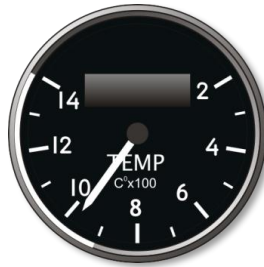
Figure 32. Fan Turbine Inlet Temperature Indicators (FTIT)
