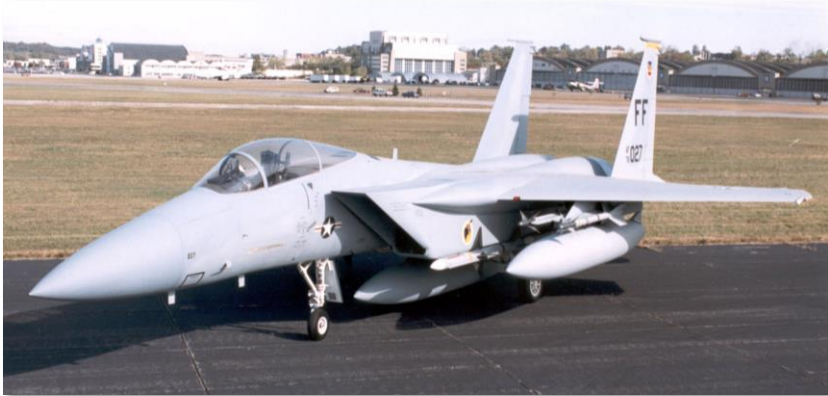
Figure 9: F-15A with AIM-7 and AIM-9 missiles
