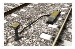
The PZB system incorporates in-cab signalling, this is where the control desk has indicators, alarms and buttons that will react according to the signalling status on the railway. The mechanism by which this works is a series of "balise" magnets placed on the side of the track. An example of one of these magnets is shown in the image on the left.
