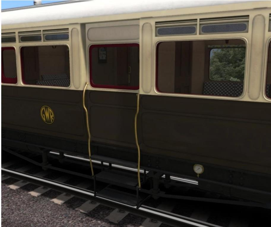
The autococh has a set of steps at the passenger doors. These were operated by the guard using a lever inside the porch when the train stopped at ground level platforms. These halts were added to branch lines when a quick and cheap pick up/drop off stop was required rather than a full station with raised platforms.
