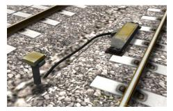
The PZB system incorporates in-cab signalling. This is where the control desk has indicators, alarms and buttons that will react according to the signalling status on the railway. The mechanism that is involved includes a series of balise magnets which are placed on the side of the track. An example of one of these magnets is shown in the image on the left.
