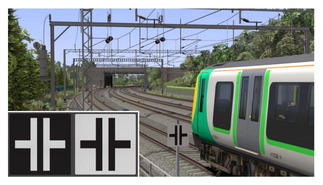
Neutral sections are marked for drivers with signs as shown above. A white-on-black sign marks the approach to the neutral section, giving drivers time to prepare the train to pass it. A black-on-white sign marks the beginning of the neutral section itself.
