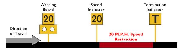
Temporary speed restrictions are normally put in place when engineering works and track maintenance is taking place. These temporary speed restrictions are advised in the drivers' weekly operating notice and in this simulation are advised in your scenario briefing. The normal sequence of trackside signage is shown above.
