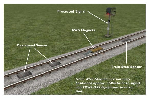
There are two pairs of grids mounted between the running rails. Both pairs consist of an 'arming' and a 'trigger' grid. The first pair, the Overspeed Sensor (OSS), are positioned on approach to the protected signal. The other pair of grids are mounted back to back at the signal location, and these form the Train Stop Sensor (TSS).
