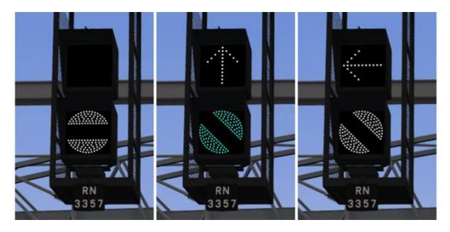
Standard banner repeater signals indicate whether the signal ahead is displaying a proceed aspect or is at danger. Modern fibre optic banner repeating signals, as shown above, consist of a rectangular unlit black background displaying a white circle with a black bar. In certain situations they can also illuminate in green to show that the signal ahead is also displaying a green (clear) aspect.
