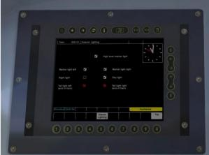
The TMS provides information about the current state of the train. Above left it shows a current train formation of 8 cars and an analogue clock. Above right shows the exterior lighting page that provides the current state of the headlight and tail light lamps (the display has also been dimmed in this image using the TMS Brightness Key).
