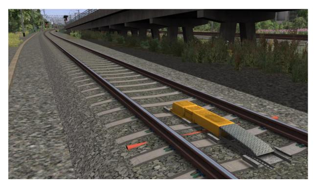
AWS is provided to give train drivers in-cab warnings of the approach to signals, reductions in permissible speed and temporary/emergency speed restrictions, and to apply the brakes in the event that a driver does not acknowledge cautionary warnings given by the system.
