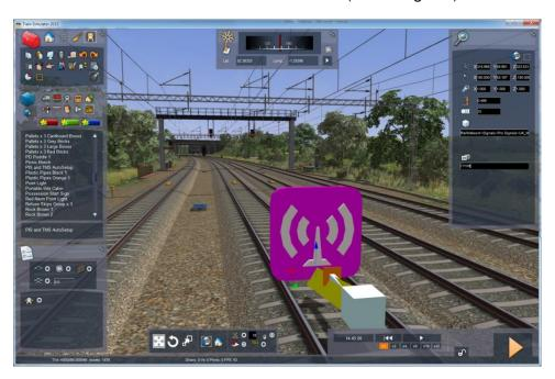
After placing a trigger where you want the event to take place you need to enter a six digit number in to the dialog box on the right of the scenario editor as shown above, then press enter to save the entry. If you need to change the number never try to edit it – delete the trigger and add a new one otherwise your changes will not be saved. The numbering system is explained below.
