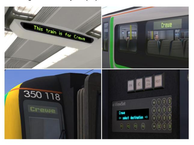
The driver can cycle through available PIS destination displays using the left and right arrow soft-keys on the PIS panel in the cabin. When active these destinations and associated messages are displayed on the PIS panel, passenger compartment overhead display, DMOS body side displays and exterior train end displays as shown above.
