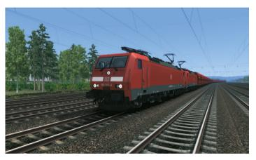
This electric loco is used for heavy freight duty.
