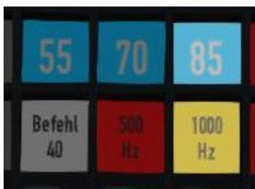
When the 1,000Hz magnet has been passed an audible alert will sound and the "85" display will begin to blink.
