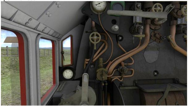
Once on the move the small ejector should be left open to maintain the vacuum at 21"Hg against leakages. The brake handle should be left in the Off position.
