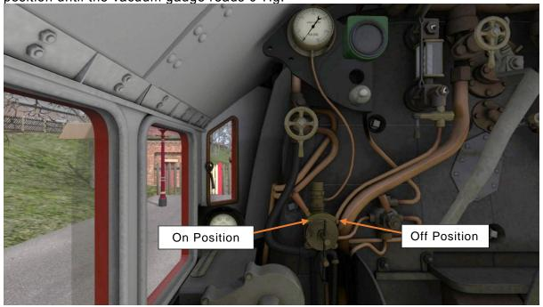
To prepare for setting off return the brake handle of the Off position. To prevent unintentional movement keep the locomotive steam brake applied (see Part 8). With the brake handle in the Off position press **P** once. Next open the small ejector and the vacuum will now start to rise.
