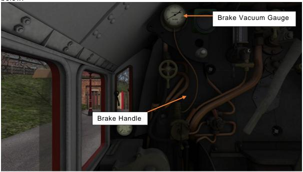
You will find the brake handle near the Off position, both ejectors shut and the vacuum partially destroyed.
