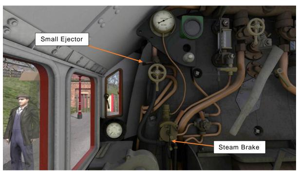
When the vacuum reaches 18"Hg the vacuum train brake is fully released.
