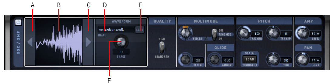
A. Previous Waveform B. Waveform display C. Next Waveform D. Name E. Load Waveform F. Phase
