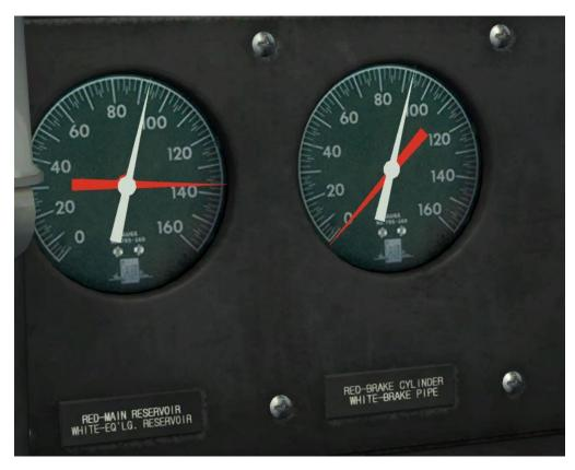
In the example above the brakes are released and both the Equalising Reservoir gauge and Brake Pipe gauge show 90psi.
