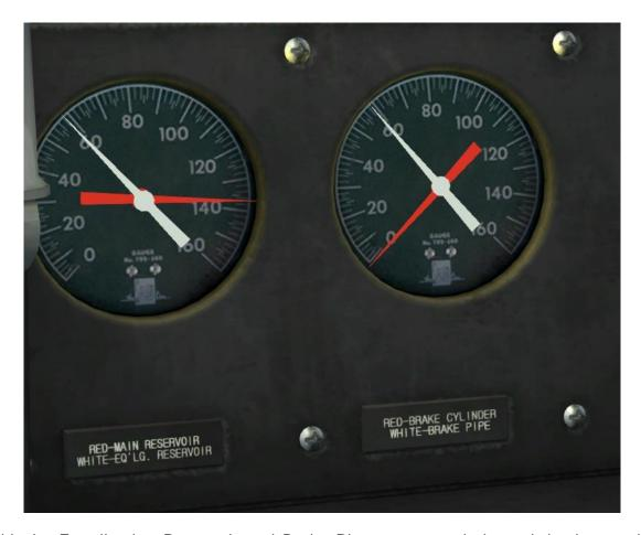
With the Equalisation Reservoir and Brake Pipe pressures balanced the locomotive Independent Brake may be 'Bailed Off' (by moving the Independent Brake lever backwards slightly). This practice removes the danger of the locomotive skidding under braking. In the above picture the locomotive brakes have been Bailed Off with the Train Brake application as before.
