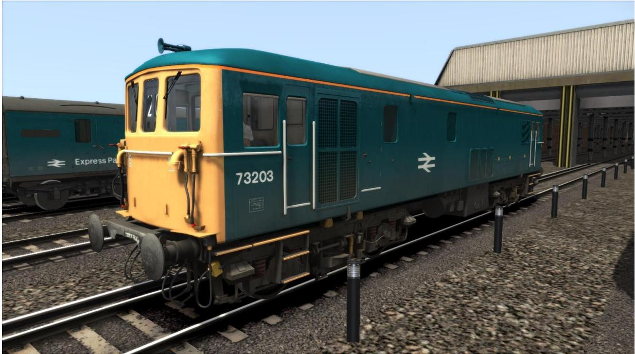
The Class 73 is an electro-diesel locomotive designed as part of the British Railways 1955 Modernisation Plan.
