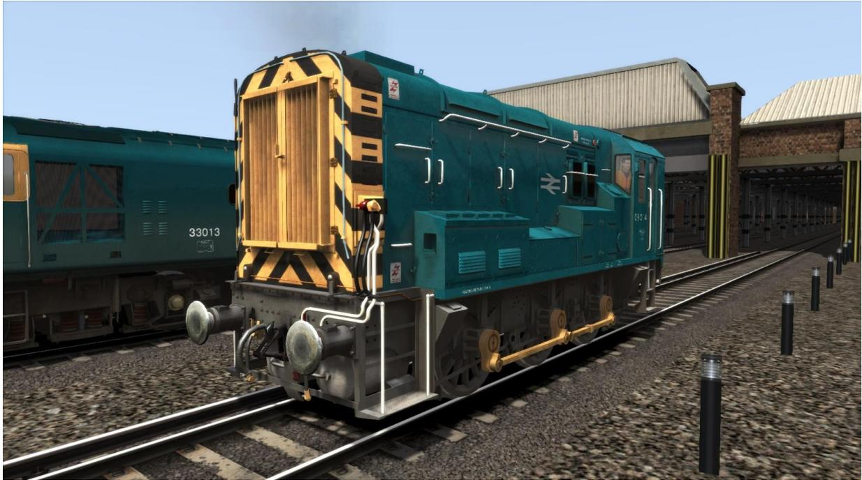
The British Rail Class 09 is a class of 0-6-0 diesel locomotive designed primarily for shunting and also short distance freight trips along branch lines.
