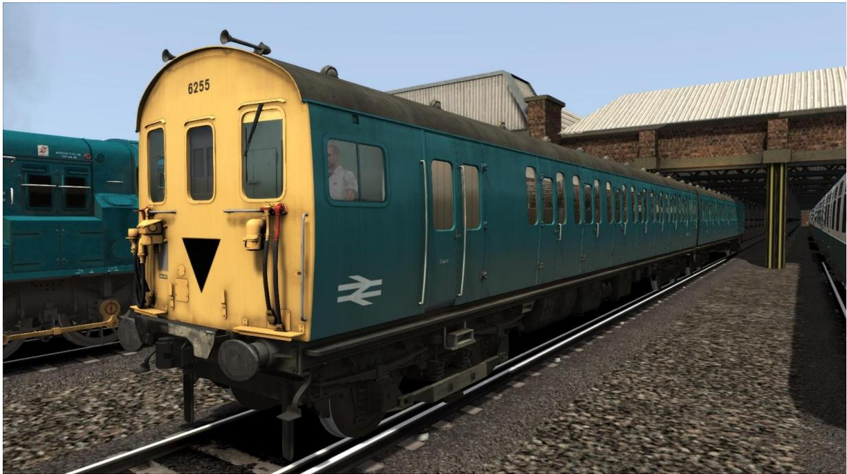
British Rail Class 416 (2 EPB) electric multiple units were built between 1953 and 1956. They were intended for inner suburban passenger services on London's Southern Electric network. There were two subclasses of Class 416: Class 416/1 to an SR design on salvaged 2 NOL underframes, and Class 416/2 to BR's Mark I coach design.
