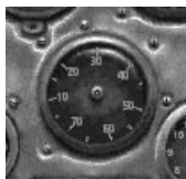
Manifold pressure gauge
