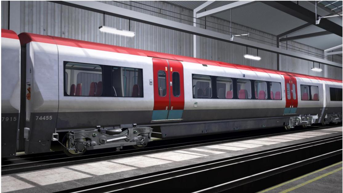
**MSO (Motor Standard Open)** - has an unpowered bogie, fitted with shoe-gear, at the number 1 end, and a motor bogie at the number 2 end. Equipment includes Brake Reservoir, Brake Module, Propulsion Inverter, Auxiliary Converter and battery box.
