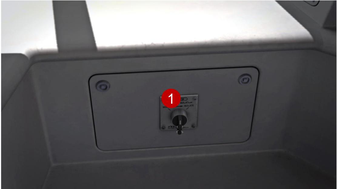
1. Train Protection and Warning System Temporary Isolation Switch
