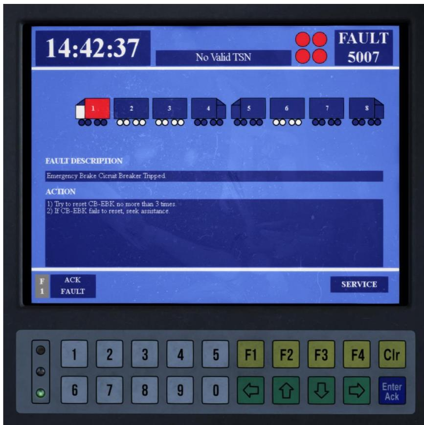
If a fault develops, an audible warning will sound and the TMS screen will display information about the fault until the driver acknowledges it by pressing the **F1** button on the keypad.
