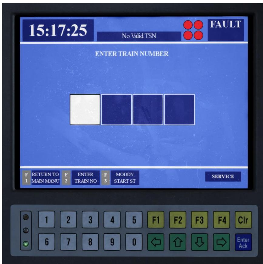
By pressing **F2** on the TRAIN STATUS page, the driver can access the train service number page, which is used to set the active destination. Available service numbers (TSNs):
