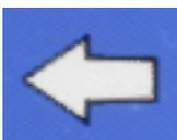
The white arrow indicates the direction of travel, based on the position of the driver's direction selector.
