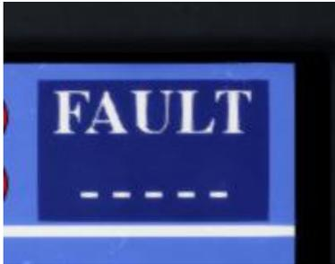
If a fault is detected by the TMS, the fault number will be displayed on the top right of the screen. If no number is displayed, there is no fault.
