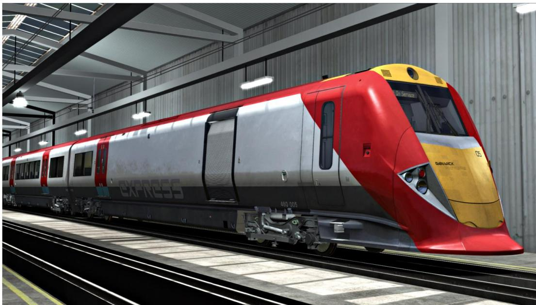
**DMLFO (Driving Motor Luggage First Open)** - usually situated at the London end of the formation. The luggage compartment is locked permanently out of use unless required under exceptional circumstances, it can only be accessed through the cab or roller doors when unlocked using a porter's key (note, this is not a BR1 or 'T-key'). The roller doors are not operable in this simulation.
