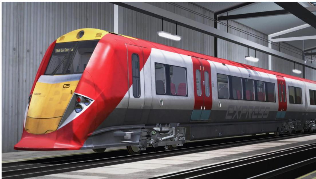
**DMSO (Driving Motor Standard Open)** - functionally and mechanically identical to a Driving Motor Luggage First, with the luggage area substituted with 60 seats in a 2 + 2 configuration.
