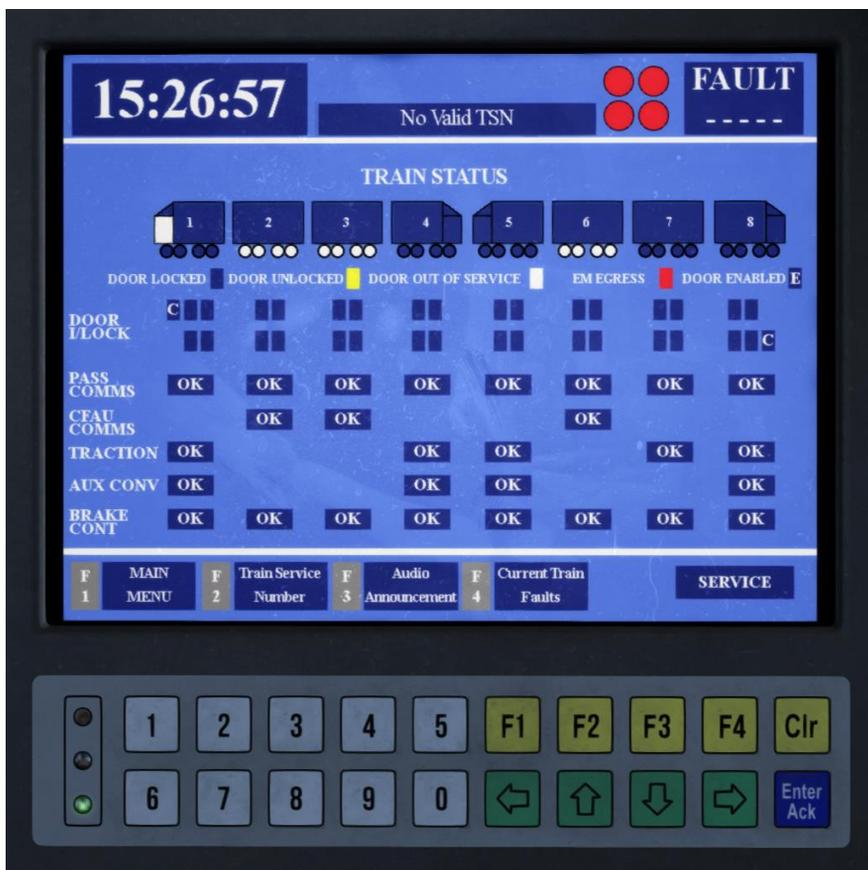
Once logged in, the TRAIN STATUS page will appear. This allows the driver to check the status of many critical and important systems, including door interlock, traction motors, and brake continuity wires.
