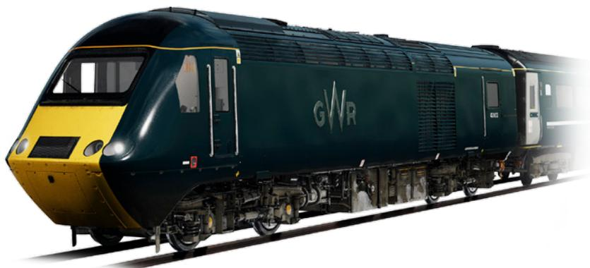
The British Rail Class 43 is an icon of high speed travel in the UK and currently holds the World Speed Record for a Diesel-Powered train. However, they did not start life as Class 43s but were in fact designated as multiple units classified, under TOPS, as Class 253 and Class 254. Designed in the latter part of the 1970s, the “HST” (short for High Speed Train) as they would be lovingly referred to by fans of the class, they became something quite unexpected.
