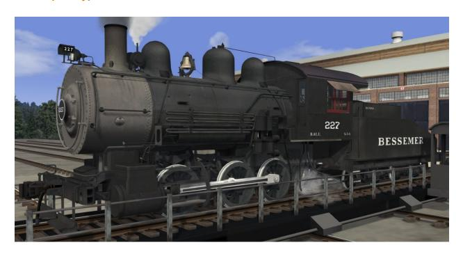
During the turn-of-the-century era, the B&LE owned eleven coal-fired "Six-Coupled" 0-6-0 steam locomotives. The final seven 0-6-0s, modeled here, were built by Baldwin beginning in 1909. They were used primarily for switching duty in the yards, assembling ore and coal trains. Though the Baldwin delivery included a sloped-back tender, a conventional tender is also included for variety.
