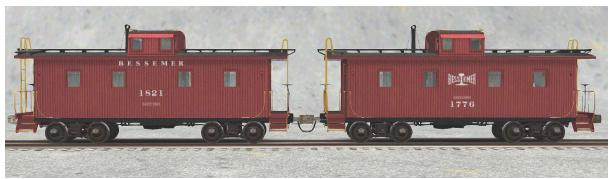
No train of the 1920s is complete without a caboose. This wooden body four-axle caboose, built in the B&LE's own Greenville shops, is a typical example of a caboose from that era.
