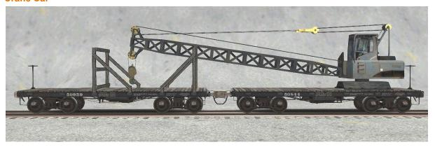
A small maintenance-of-way and wreck crane for lighter duties. Built on top of an old 30 ft flatcar frame and matched with a similarly home-built boom car.
