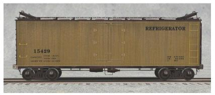
This is a wood-and-steel body icebox refrigerator car, used to transport agricultural produce and other perishables. Blocks of ice can be filled into boxes below the four hatches on the roof, keeping the interior of the insulated car cool for many hours.
