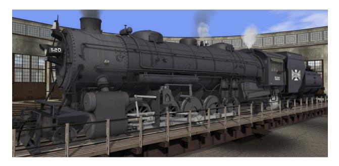
The B&LE owned 25 coal-fired "Santa Fe" 2-10-2 steam locomotives. All were built by Baldwin beginning in 1916, including 19 D-1-A class, as modeled here. These locomotives were designed for tractive power rather than speed, hauling heavily laden ore and coal trains over the full route. The locomotives were equipped with a Street mechanical stoker, and a Vanderbilt-style tender. The "Bessemer" labeled tender is provided in both railhead (shown) and block-lettered formats.
