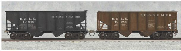
Hoppers are the main aggregate haulers on our route. Mainly used in coal and ore traffic, these cars also see service transporting gravel and limestone. Three B&LE liveries are included, the earlier all-black paint schemes and the later orange paint that the railroad adopted to combat the heavy decay inflicted on those cars by the iron ore.
