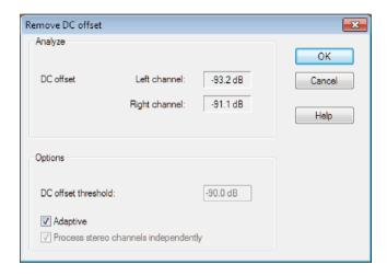
In **Adaptive** mode (preset) a variable, rather than constant, DC voltage is emanated. On technical terms, all frequencies under 10 Hz are used as DC. If "Adaptive" is deactivated, a constant DC is emanated. You can enter a minimum **DC offset threshold**, which indicates where DC offset removal will kick in. You can also edit stereo channels together to reduce computing time.
