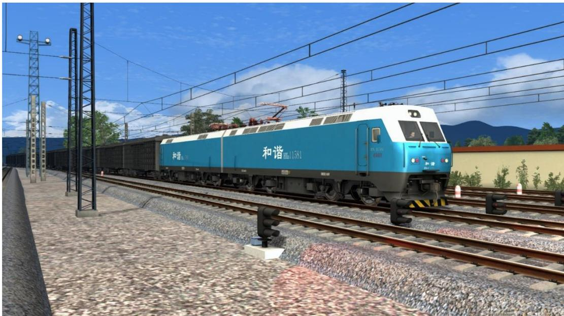
The HXD1 locomotive, a new heavy load freight locomotive is available to use on the mainline.
