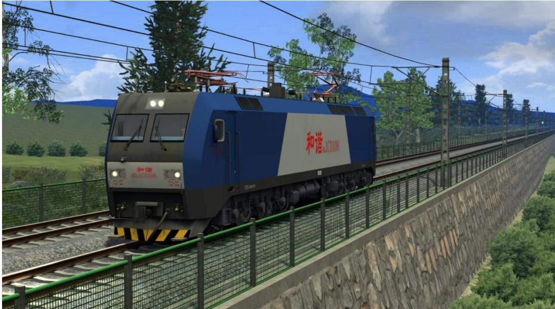
The HXD1C locomotive is a high-power AC drive six-axle electric locomotive with a power of 7200 kW. It was designed with its own set of fully independent intellectual property rights. 90% of its components are made in China. The locomotive's design makes use of nine main technology patents, being the locomotive's assembly, carbody, bogie, traction transformer, traction converter, network control system, traction motor, driving device and brake system.
